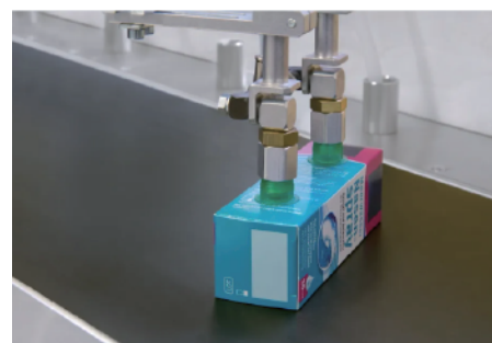
*Examples of packaged workpieces handled by HSXA suction cups
