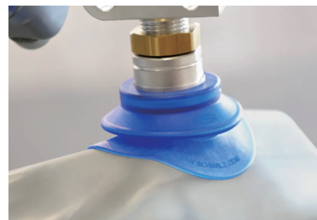
*Examples of HXF suction cup handling curved workpiece surfaces
